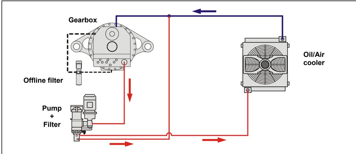
When the optimum operating temperature is not reached yet, a thermal bypass shorts the circuit and conducts the pre-heated oil back to the gearbox. As soon as the optimum operating temperature is exceeded, the active oil/air cooler starts and cools down the oil. Each cooler is additionally equipped with a fan, which is switched on or off depending on the oil temperature.
